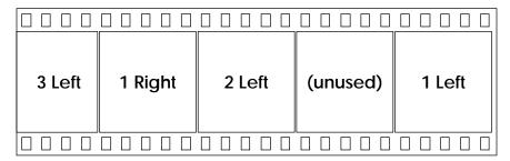
In this format, the film advances two frames for each exposure. This results in an unused exposure at the beginning and end of the film. The extended film sequence is 1L-unused-2L-1R-3L-2R-4L-3R- etc.
