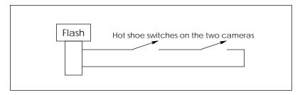
This has the effect of ANDing the two camera hot shoe switches, causing the flash to not fire until both shutters are closed. Kevin cautions: "It was a little tricky getting the wires right, and I got zapped a few times because I forgot that the outer connections of cameras' pc-jacks are already connected via the bodies and aluminum plate they're mounted on".
