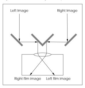
A similar arrangement is built into a viewer used to view either the slides or prints produced. (The images may also be free-viewed, cross-eyed method). Equipment currently available new using this principle includes the Ukrainian-made SFK-1 beamsplitter, the Franka beamsplitter, a 35mm attachment made by Pentax, and the Loreo camera.
